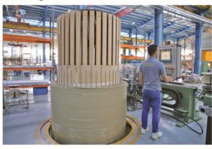
Horizontal winding machines are used to wind layer, helical and regulating windings with height up to 1,900 mm and weight up to 4,000 kg.
