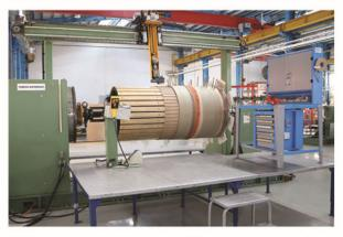
All those winding machines operated by a PC-supported machine control system which also allows transfer of winding data to the machine through the company network.
