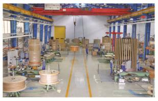
The winding process is closely monitored by control system. The winding program inside can calculate all stop points and automatically executes the bending. Vertical winding machines are specially designed to wind transposed disc windings with single or multiple flat conductors with height up to 2,200 mm and weight up to 14,000 kg.
